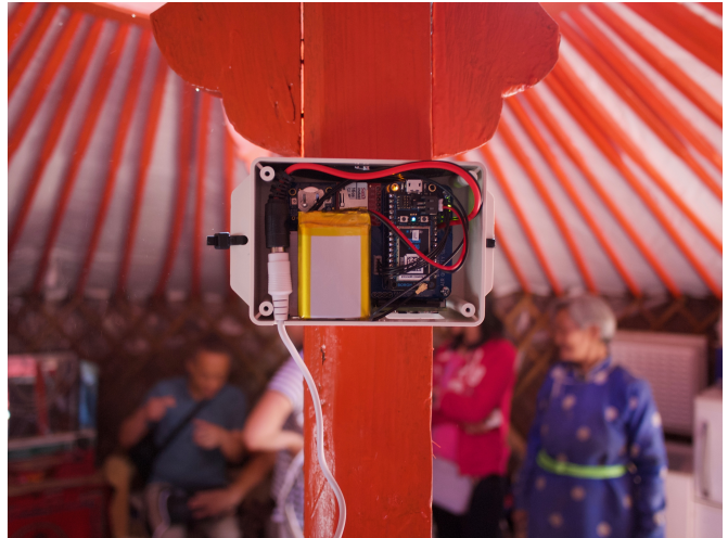
Fig. 2. Our air quality sensor, with its cover off, deployed in a ger.
